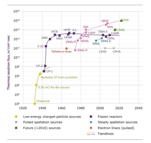
Figure 3. Thermal neutron sources fluxes
