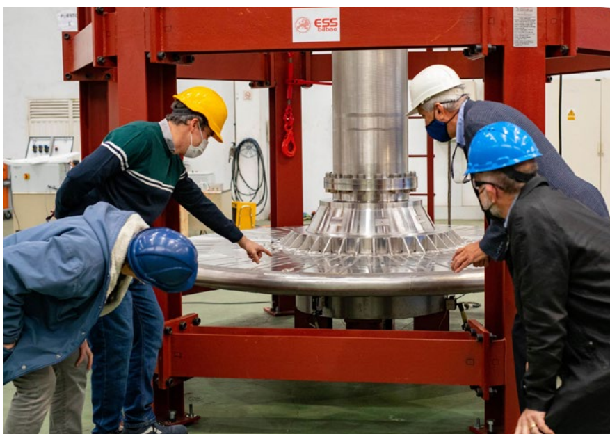
Team members from ESS and ESS Bilbao inspect the target wheel during final testing before its onward journey to Lund
